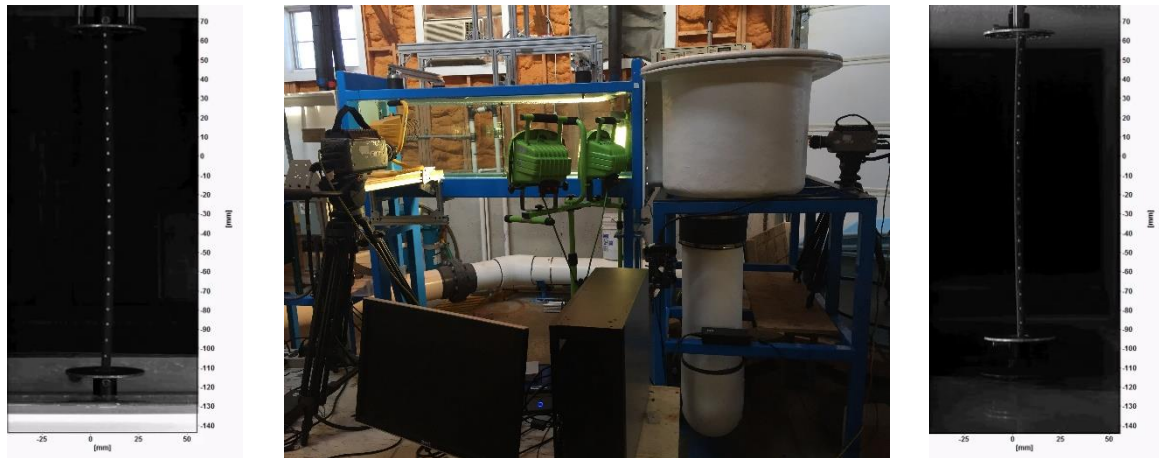
Fig. 3. Experimental set-up in flow channel. Left image: In-line camera view. Center image: Flow channel set-up. Right image: Cross-flow camera view.
